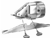
assembling side guide with two wing screws
